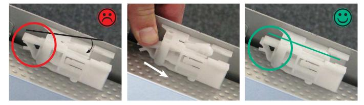
Before assembly check that both latches are in 0-position. The latching element can shift out of 0-position following either incorrect assembly or disassembly.
