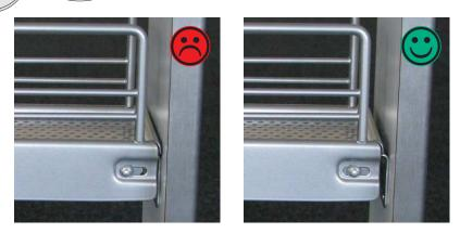
If the gap between the front panel and the fitting is less than 4 mm, the fitting cannot be pushed far enough into the unit to engage with the slides.
