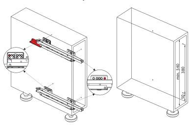
The slides must be fitted parallel to each other. In addition, it is important that the dimension of 380 mm is maintained exactly.
