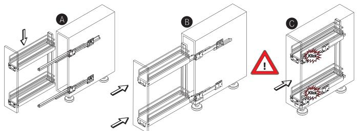
Pull slides fully out of the unit. Push fitting onto slides and then back into the unit. An audible click means that the slides have engaged with the fitting.
