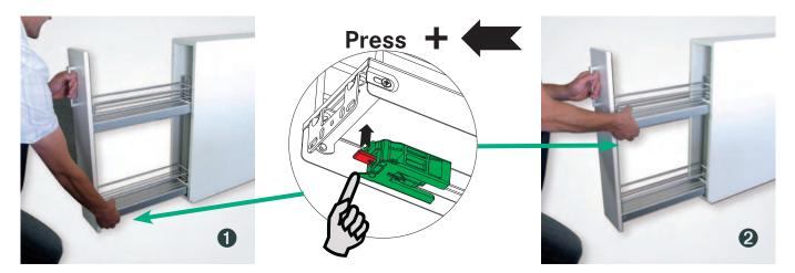
Pull out front panel with fitting until clear of unit (approx. 10 cm). Then lift off.
