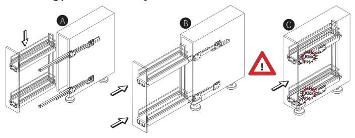
Pull slides fully out of the unit. Push fitting onto slides and then back into the unit. An audible click means that the slides have engaged with the fitting.
