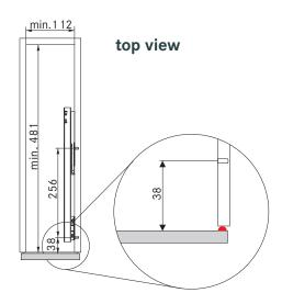
If the sealing lip/limit stop are not taken into account, the slides will be attached too far into the unit and cannot engage with the fitting.
