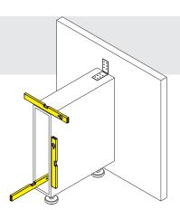
The slides must be fitted parallel to each other. In addition, it is important that the dimension of 380 mm is maintained exactly.
