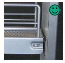
If the gap between the front panel and the fitting is less than 4 mm, the fitting cannot be pushed far enough into the unit to engage with the slides.
